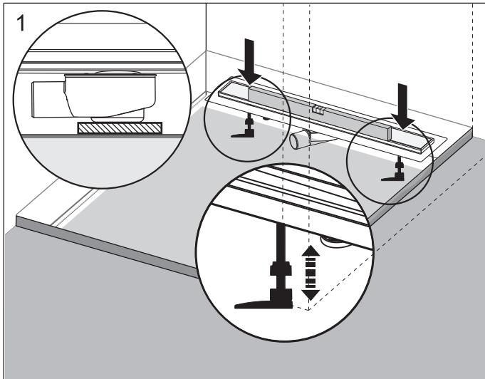
EN / Place the drain on the floor and secure it by fixing the feet into the floor (not included). Use a construction level to adjust the height of the feet. The metal grid must be aligned with the level of the finished floor.
