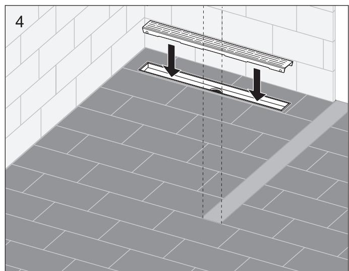
EN / Complete the installation of the gangway: install the mesh to catch fine debris, then the grate.
