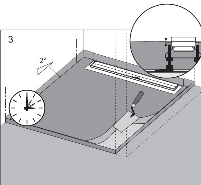
EN / Screeed the floor up to the drain body. The slope of the housing must be at least 2° towards the drain. Apply a layer of waterproofing surface sealant according to the manufacturer's recommendations. After drying, apply waterproofing tape (not included). Then finish the floor with the chosen material.
