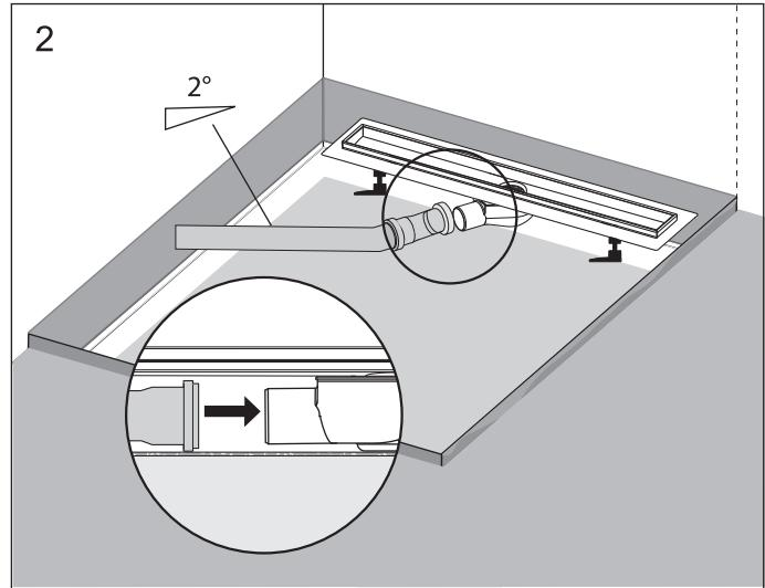
EN / Measure the length of the sewer pipe running from the riser pipe to where the drain is to be installed. For each meter of length, the slope of the pipe should be 1.5-2 cm (or 2°). Connect the sewer pipe with a rubber sealing ring to the outlet of the drain for a tight seal.
