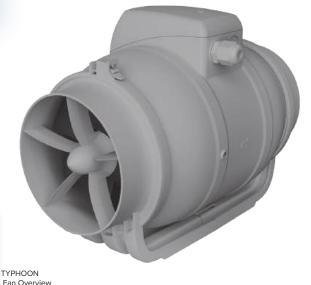
Mixed-Type Axial Duct Fans designed for supply and exhaust ventilation systems in industrial, commercial, and residential buildings. The central removable unit, which includes the motor, impeller, and terminal box, is secured to the ducts with clamps. This significantly simplifies maintenance.
