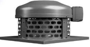
Roof fans of the ERF range are designed to maintain air exchange in residential and commercial buildings and are used to remove polluted air. The roof fan with horizontal air discharge is equipped with a motor with reusable overheating protection and automatic restart. The insulation class of the electric motor is F. Fans are installed on a mounting cup or ventilation shaft in a horizontal position on roofs of any type.
