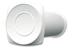
The KP supply valve is designed for fresh air supply in premises with forced ventilation systems. The supply valve is an insulated air duct with complete sound and heat insulation. The G3-class filter capturing >80% of particles >0.4 microns (effective dust retention). Indoor side features an adjustable damper for precise airflow control and the outdoorside is equipped with one of the foor facade air diffuser options (model-dependent).
