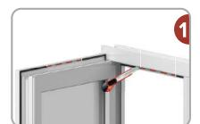
Remove the sealant from the frame and the casement window at the length of WV (350 mm).
