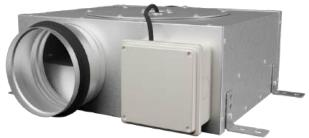
exchange in supply and exhaust ventilation systems in rooms with a shortage of mounting space. STELS have the lowest mounting height\*. They are installed in the channel in any position. The single-phase ball-bearing motor with an external rotor has thermal protection with automatic restart. The connection is carried out in a sealed terminal box. Rubber seals on the flanges simplify installation and ensure reliable sealing.
