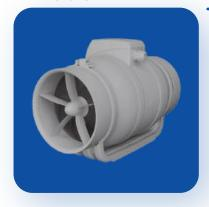
Inline fans are used in exhaust and supply ventilation systems for residential, commercial, and industrial facilities. These compact units install directly into ducts and are classified into two types: axial and centrifugal. Axial models deliver high airflow velocity at low static pressure, while centrifugal fans excel in high-pressure differential applications.
